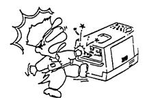
■ **NEVER** touch output terminals during operation. This is extremely dangerous. Always stop the machine when contact with the output terminals is required.
